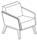
Chair with Upholstered Back W29" D30.25" H31.5" Seat: W22.5" D20.25" H18.5" Arms: H26.25"
