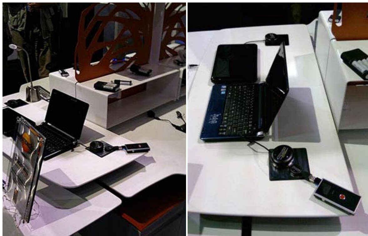
Kimball Office desking with embedded WildCharge grommet; photos by Aly Saxe.
